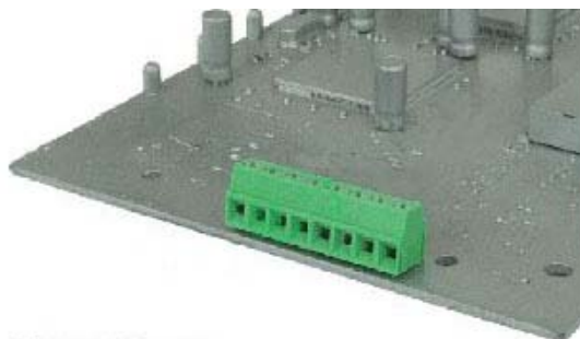
Figure 6. Terminal 1 for VPS, TEC+ and TEC- ports
